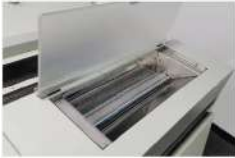
Flip top powder box, simple operation, convenient to add powder.
