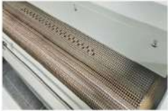
With belt system, you can cut off files, while printing. Since the film is fed by air suction system. And cut production at the same time.
